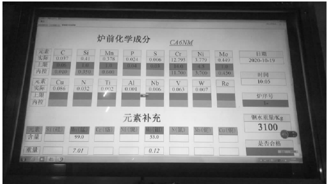
图 5 熔炼车间炉前加料系统大屏幕 Fig.5 Large screen of feeding system before furnace in the smelting workshop
